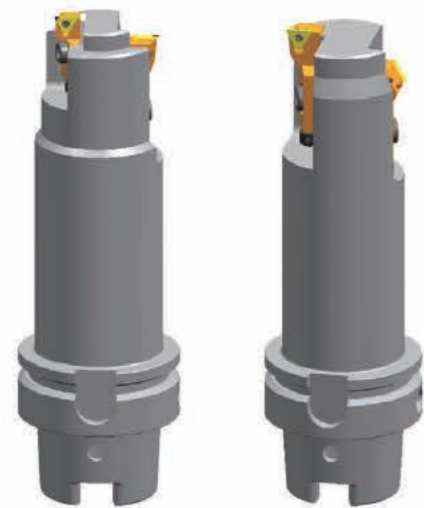
• GEAR SHIFT SHAFT LOCK HOLE BORING TOOL
