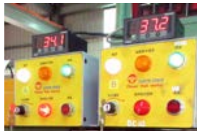
Controls require operator to use both hands.
