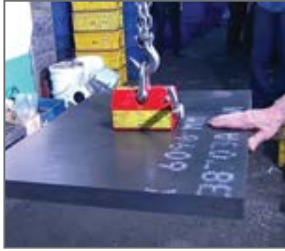
3.5 X Safety Factor above rated load capacity
