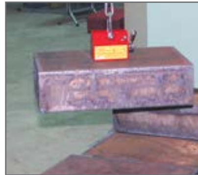
Center magnet on most workpieces to lift.
