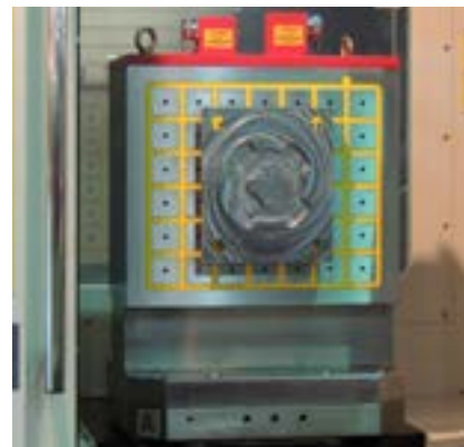
Palletized horizontal workholding chuck
