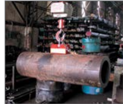
Beveled bottom surface lifts round stock.
