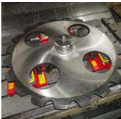
Large tooth sprocket being machined
