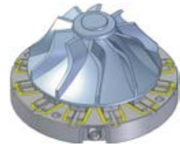
5-axis turbine blade machining
