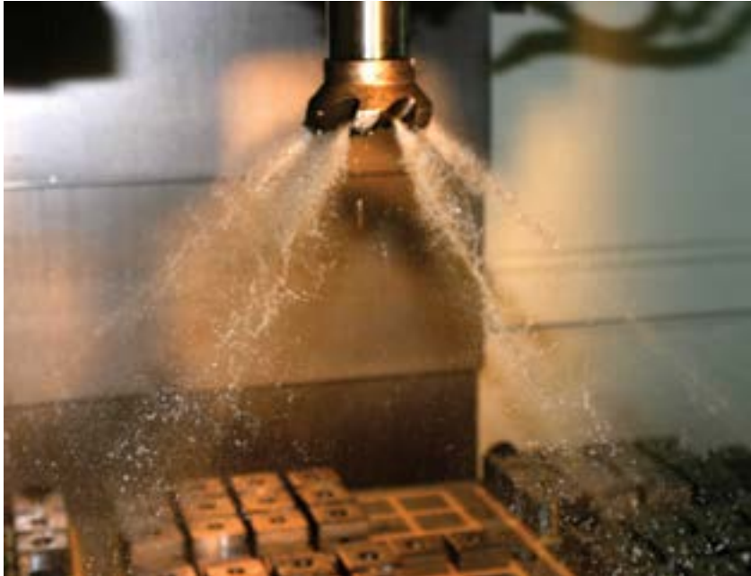
CoolBLAST arbor screw provides coolant path.
