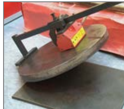
Move round or rectangular stock vertically.
