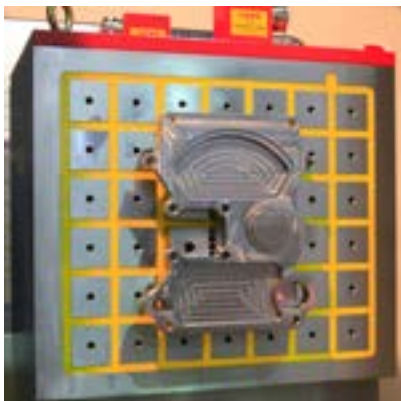
Complex part shapes - 5 sides machining
