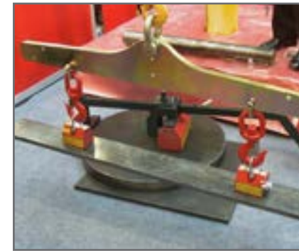
Spreader bars are used for long or very heavy loads.
