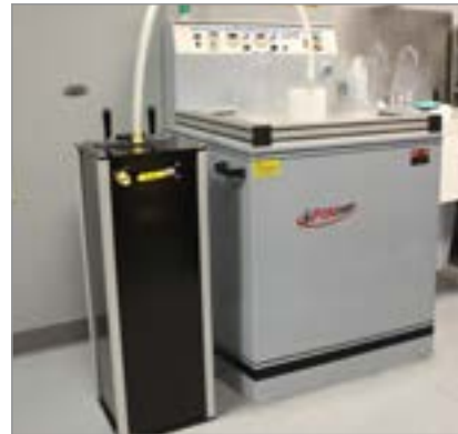
Filtration unit continuously cleans deburring fluid, minimizing machine downtime for water changes.
