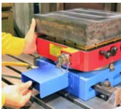
Pull knob to rotate part up to 360 degrees
