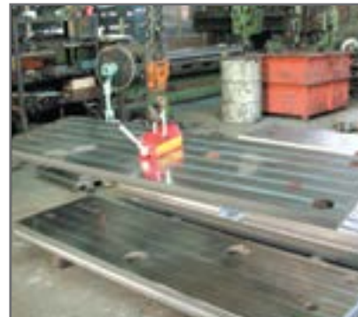
Locate magnet at balance point for lifting.
