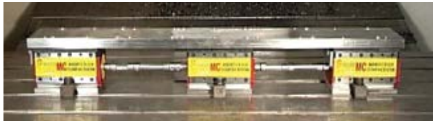
Switch-connect ECB vises to turn ON/OFF simultaneously
