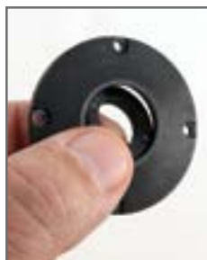
Insert Black Gold coolant ring into cap
