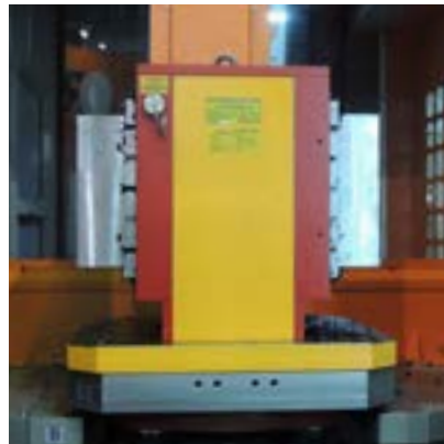
2-sided EEPM on palletized system
