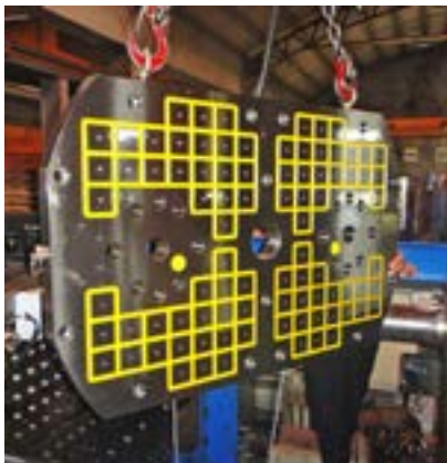
Load and install PIM magnet with bolts
