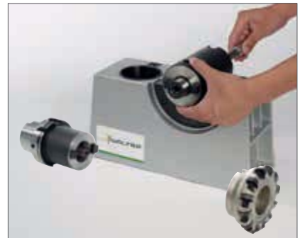
6. Screw the extension and the cutter adaptor together by hand using the socket wrench
