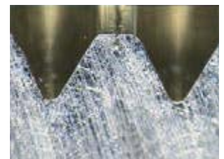
Thread profile made with a special former
