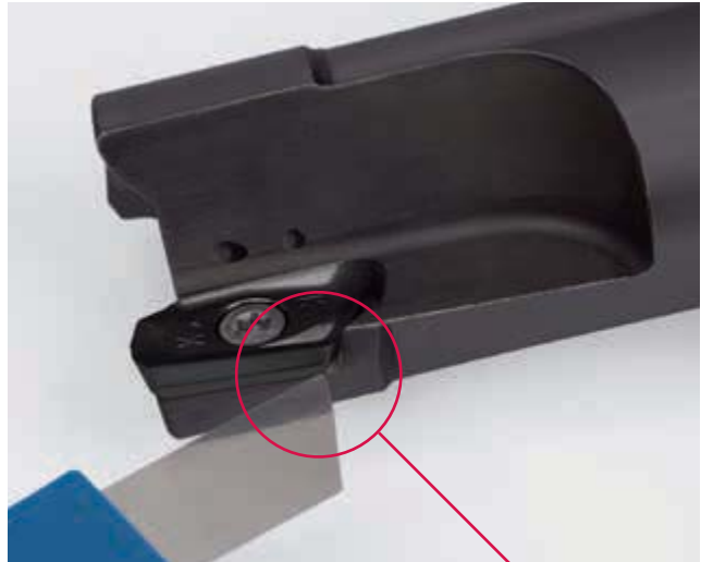
Check with 0.01 mm spacer
