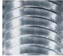
Smooth surface due to excellent lubrication
